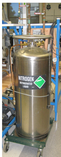
Figure 8: Liquid Nitrogen Tank Click here to see larger picture
