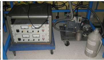
Figure 3: Magnet Power Supply & Vacuum Pump with Transfer LN-2 Dewar Click here to see larger picture
