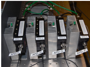
Figure 13: Fiber optic cables in to APDs
