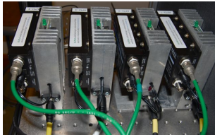
Figure 12: Power in and data out APDs
