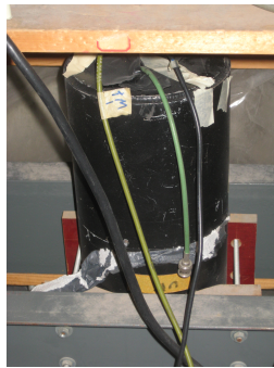
Figure 3: Close up of the black base of the top photomultiplier tube found in room 275. See larger image here
