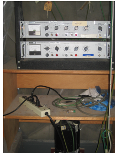
Figure 2: High voltage power supplies for top & bottom PMTs with the black base of the top PMT shown. See larger image here
