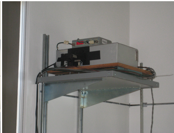
Figure 2: Low Light Diode & Chopper source box on NW wall Click here to see larger picture
