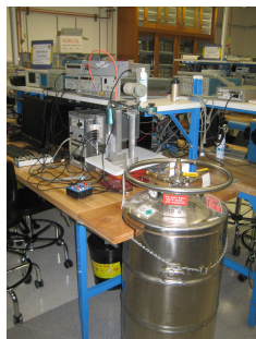
Figure 5: Liquid Helium Dewar Click here to see larger picture
