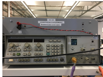
Figure 3: Power Supply, Sweep Oscillator, and RF Plug-in Click here to see larger picture
