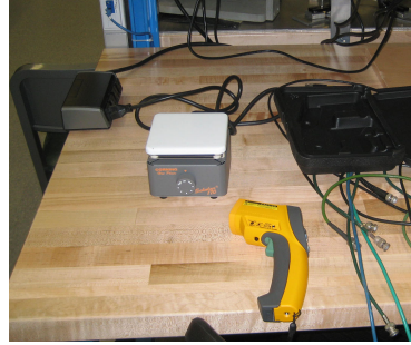
Figure 7: Hot Plate for heating points and IR Temperature meter Click here to see larger picture
