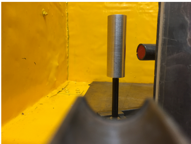
Figure 11: Incorrect shield placement. The detector is not completely blocked from the source.
