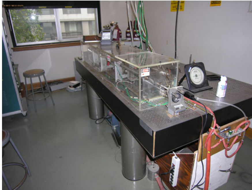
Figure 16: Room layout and air table for the laser system.
