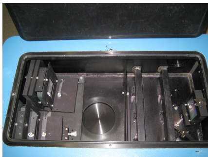
Figure 2: Monochromator Interior Top View Click here to see larger picture
