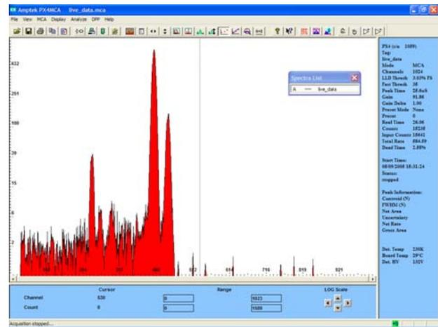
Figure 3: Acquisition spectrum for an  $^{55}\text{Fe}$  source.
