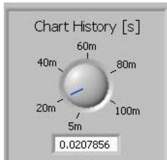
5ms is generally faster than the period of the data so a longer period is necessary in most cases. The picture below shows only half the period.
