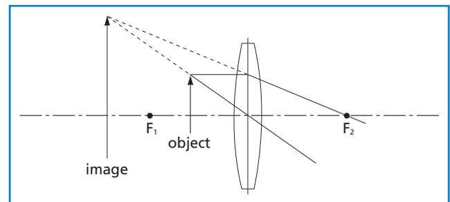
Figure 1.3 **Example 2** ( $f = 50$  mm,  $s = 30$  mm,  $s'' = -75$  mm)
