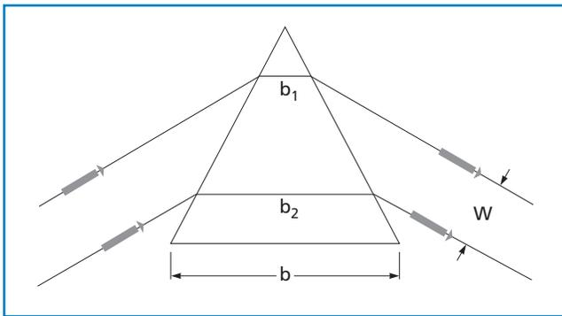
Figure 1.41 **Ray path lengths of a prism at minimum deviation**
