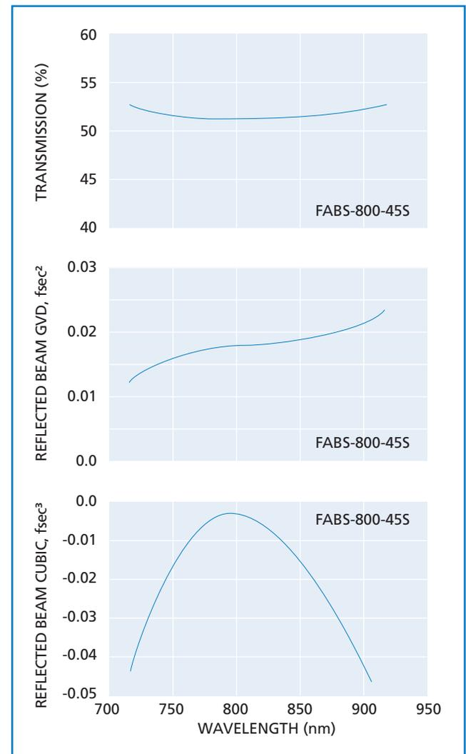
Figure 1.69 Transmission characteristics for FABS series polarizers with  $s$ -polarized light
