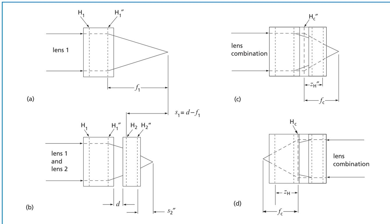
Figure 1.8 Lens combination focal length and principal planes
