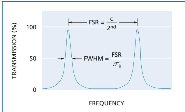
Figure 1.58 **Transmission characteristics of a Fabry-Perot etalon**
