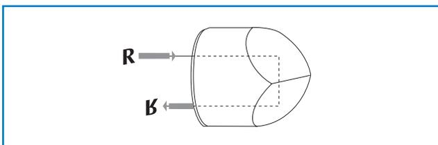
Figure 1.45 **Porro prisms retroreflect and invert the image**
