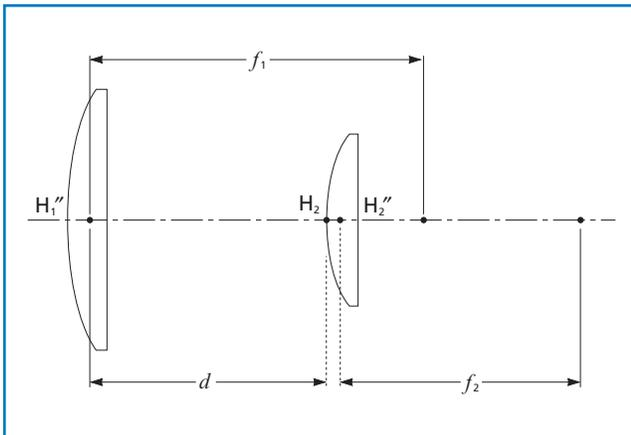
Figure 1.11 **Achromatic combinations:** Air-spaced lens combinations can be made nearly achromatic, even though both elements are made from the same material. Achieving achromatism requires that, in the thin-lens approximation,
