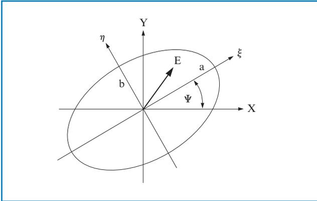
Figure 1.49 The polarization ellipse
