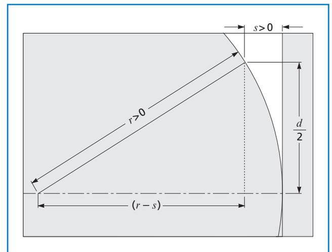
Figure 1.34 Surface sagitta and radius of curvature
