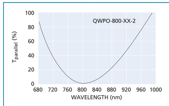
Figure 1.54 **Zero-order crystal quartz half-wave waveplate for 800 nm**
