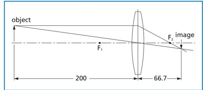
Figure 1.2 **Example 1** ( $f = 50$  mm,  $s = 200$  mm,  $s'' = 66.7$  mm)
