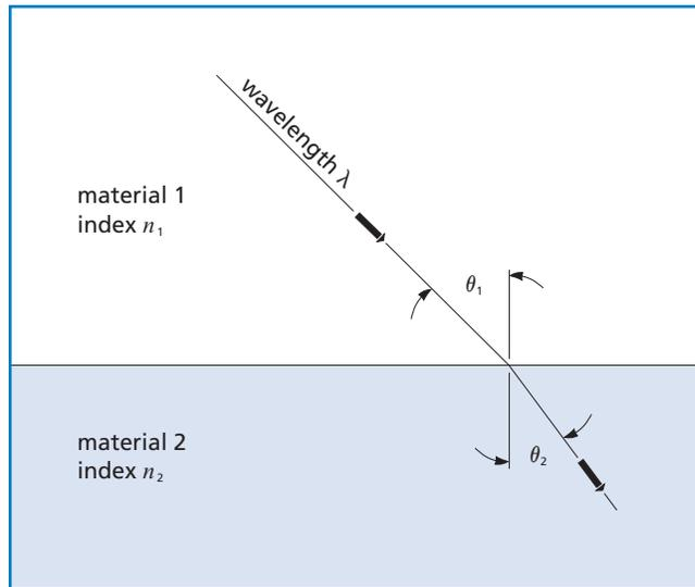
Figure 1.14 Refraction of light at a dielectric boundary
