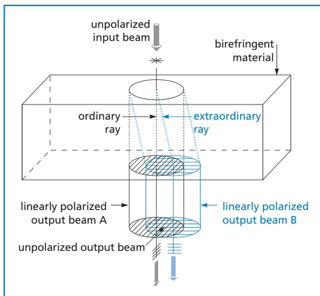
Figure 1.51 Double refraction in a birefringent crystal
