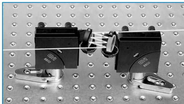
Figure 1.66 Typical optical set-up of negative GVD mirrors
