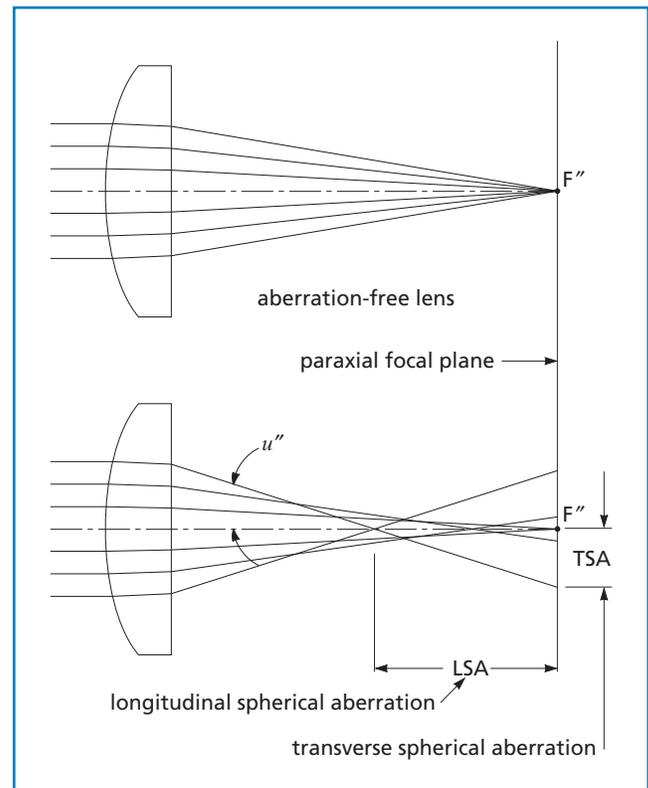
Figure 1.15 Spherical aberration of a plano-convex lens
