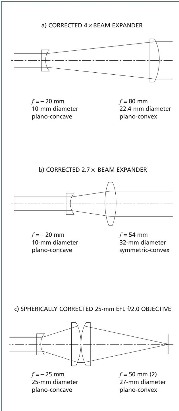
Figure 1.32 Combining catalog lenses for aberration balancing
