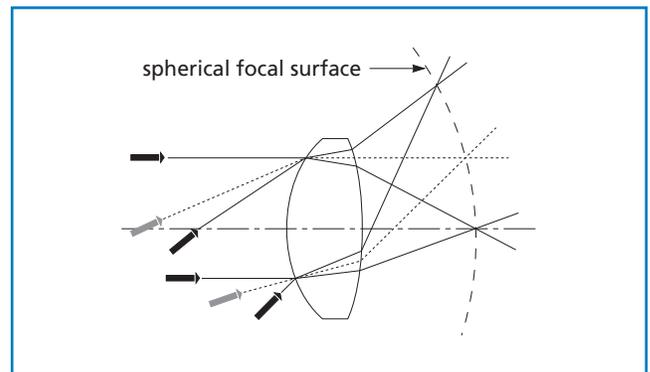
Figure 1.19 Field curvature
