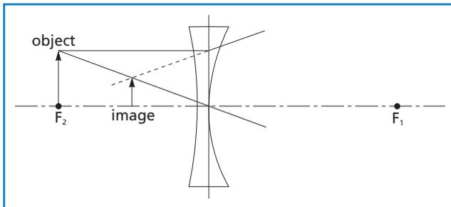
Figure 1.4 **Example 3** ( $f' = -50$  mm,  $s = 50$  mm,  $s'' = -25$  mm)
