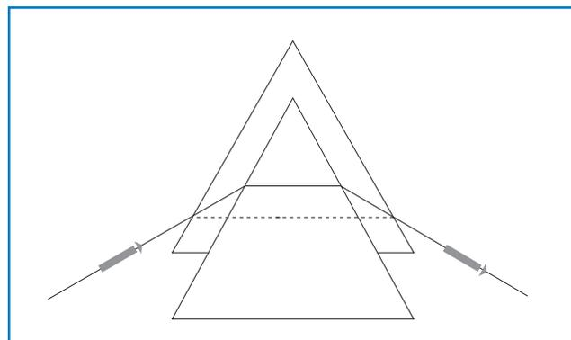
Figure 1.40 Translation of a prism at minimum deviation
