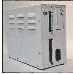
Front and back views of the TT-AFM Ebox showing indicator lights and connectors for ribbon cables and USB
