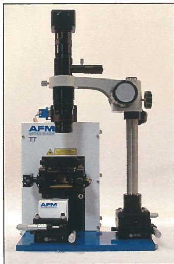
TT-AFM stage combined with the video microscope
